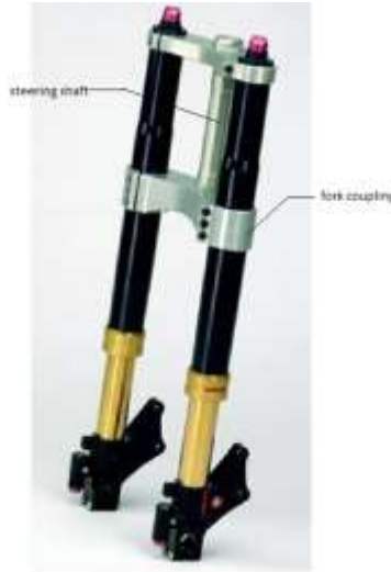
Fig 1: showing the fork coupling & the steering shaft
