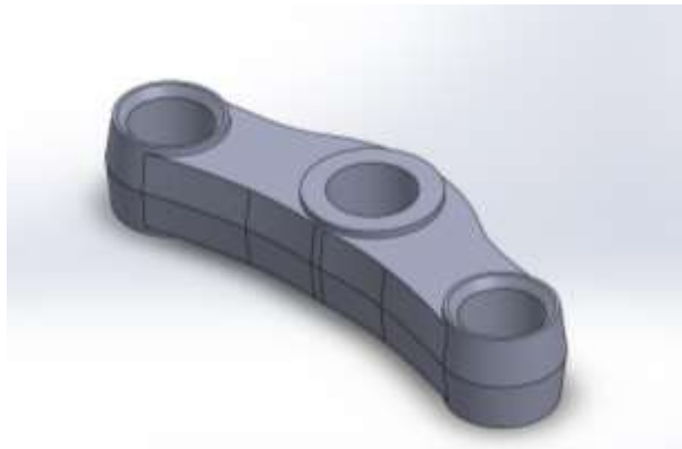
Fig 2: sample fork coupling of D=33mm, s=9mm
